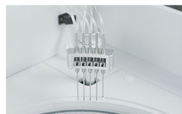
Washing Probe Independent 5-step washing system.
