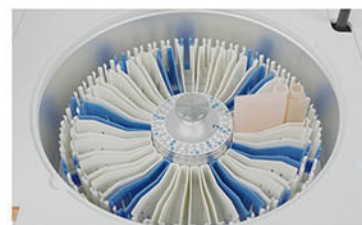
Reagent Tray 2~12°C cooling for 24 hours.
